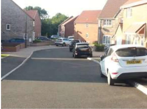
Dingley Lane, North Yate. The pavements make the road very narrow, forcing cars to be parked on the pavement. The sharp bend complies with current Government expectation on controlling vehicle speed, but is not effective in doing that. Children were very close to being run over on this bend.
